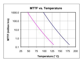
As can be seen from the MTTF numbers above, the predicted failure rate is still above 1 million hours, even at operating temperatures up to  $+110^{\circ}$  C (corresponding to channel temperatures of  $+160^{\circ}$  C). Also note that these MTTF estimates are a lower bound as the accelerated testing never resulted in 50% failures.
